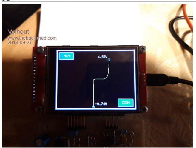
There are 2 buttons: MEM: this button stores the current waveform, and displays it in red, as a reference. This would be the waveform of the "known good" circuit. ZOOM: this button zooms in at the center, to allow more detail if low voltage circuits are probed.
